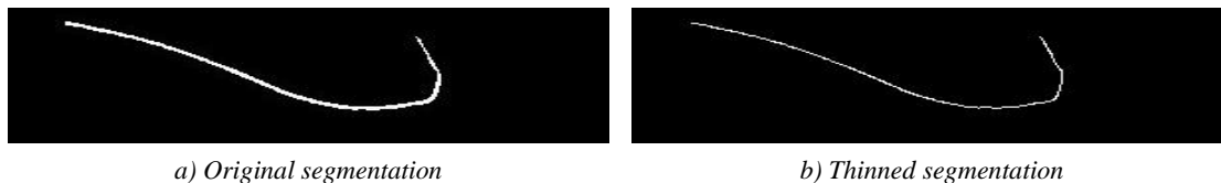
Fig. 12 : Thinning process for the catheter (zoomed in)
