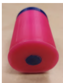
Figure 4.2: 3D printed first part consisting of; Membrane: 3D printed with Ninjaflex (material in blue color) and casing: 3D printed with PLA (material in pink color)
