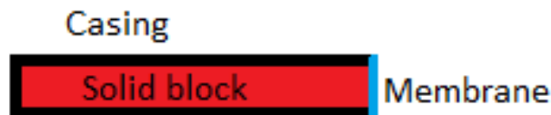
Figure 3.1: Design Sketch for solid block heating with; solid block( in red color), flexible membrane (in blue color) and casing(in black color)
