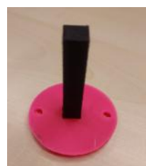
Figure 4.3: 3D printed second part consisting of; Top: 3D printed with PLA (material in Pink color) and heater: 3D printed with Potopasta (material in black color)
