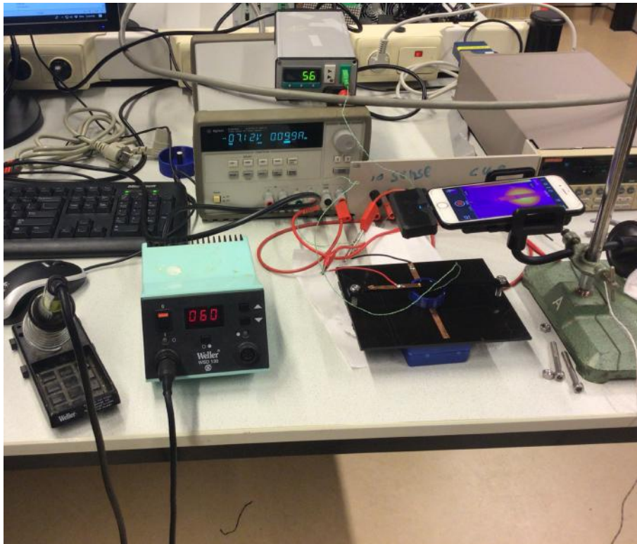
Figure 5.4: Experimental Setup consisting of; test structure filled with olive oil place on the holder, thermal camera connected to an iphone, thermocouple connected to digital multimeter, DC power supply connected to soldered wires on holder, solder iron used for calibration IR scale of thermal camera.
