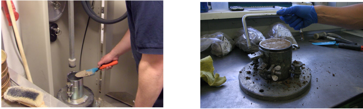
Figure 8: Snips of soil compaction test, taken from Fugro website
