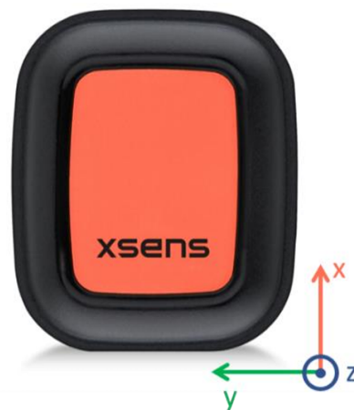
Figure 3.5: Xsens DOT sensor coordinate system [61]
