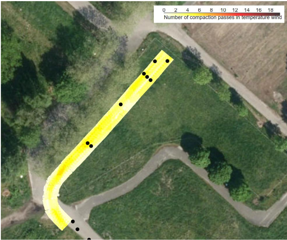
Figure 56: Number of compaction passes in TCW area A
