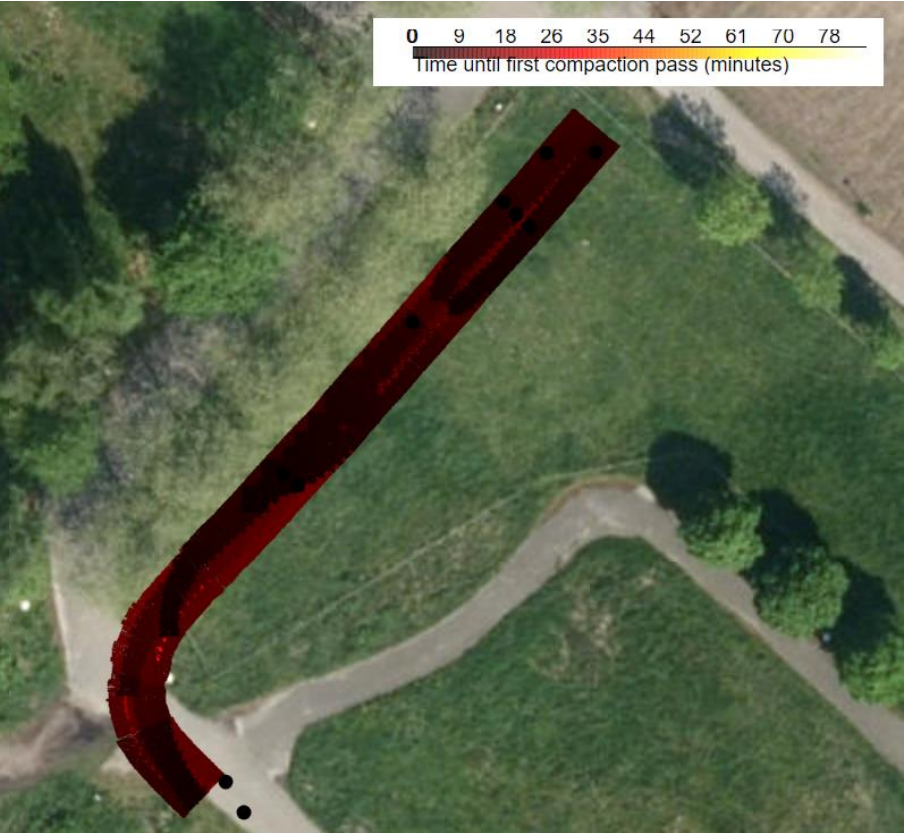
Figure 60: Seconds between paving and compacting area A
