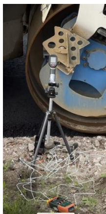
Figure 30: IR camera during a roller pass
