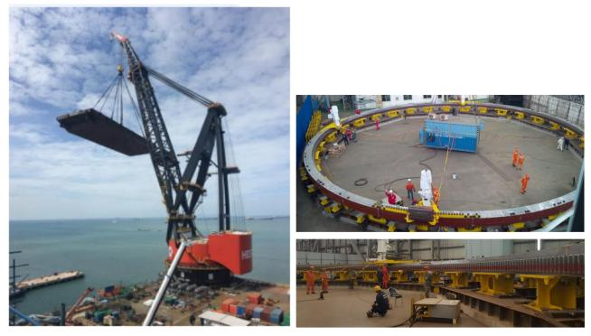
(a) Slew bearing mounted on a crane
