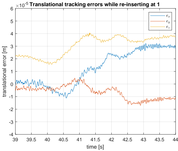
(a) Translational tracking errors while re-inserting at location 1 without touching.
