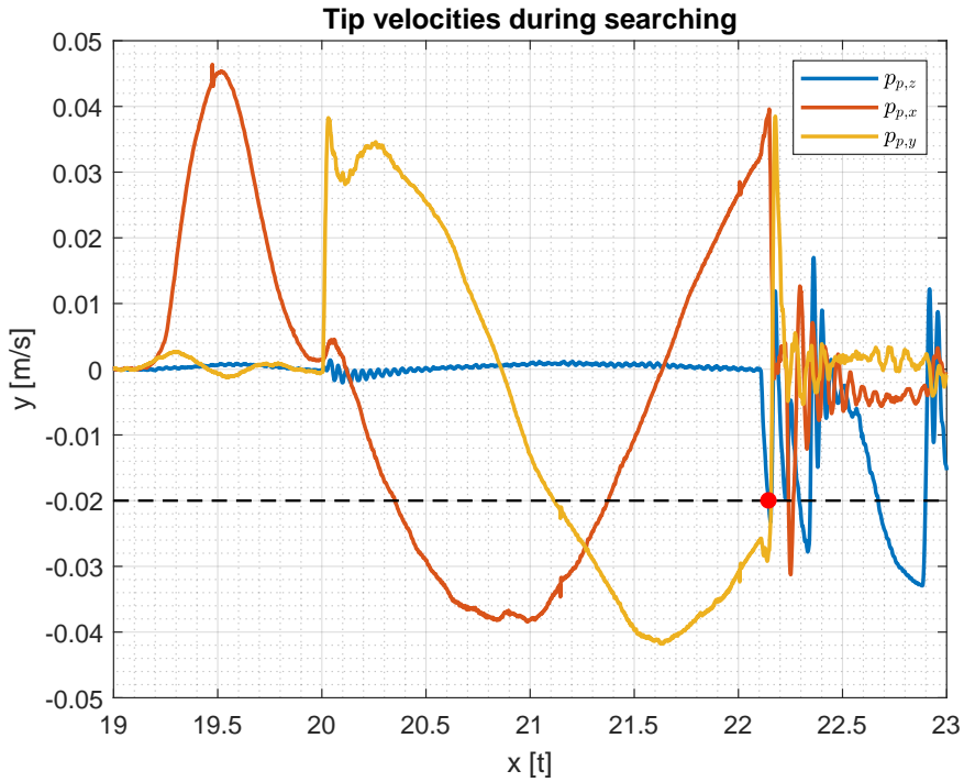
Figure 38: Reconstructed tip-velocities during searching. Dashed black line is the threshold of -0.02 \text{ m s}^{-1} , and the red dot indicates the recognition of partial insertion. A sharp peak in z-velocity is observed when the peg slips into the hole.
