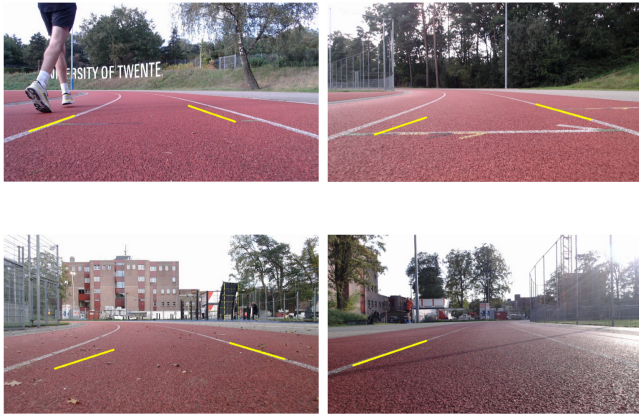
Fig. 16: Sample outputs showing false negatives (FN) represented as yellow lines
