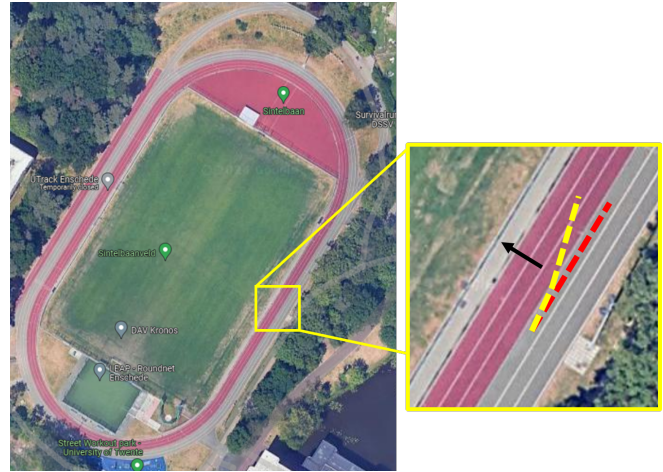
Fig. 14: Zoom-in map showing the slant direction (black arrow), absolute zero steer run (yellow dotted) and expected run (red dotted)
