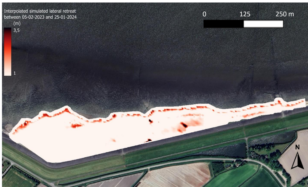
Figure 32 Interpolates simulated lateral retreat between 05-02-2023 and 25-01-2024. Redness indicate how much lateral retreat is present in that area.
