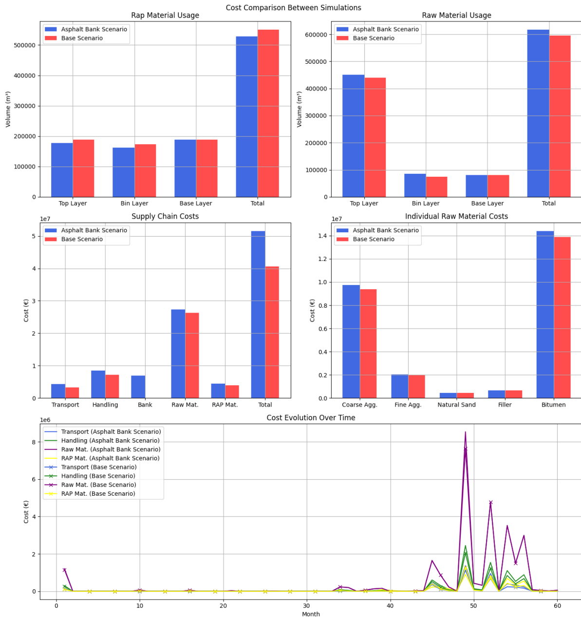
Figure 8.1: Comparing Supply Chain Cost and Raw Material Usage for the Current Supply Chain With and Without an Asphalt Bank.
