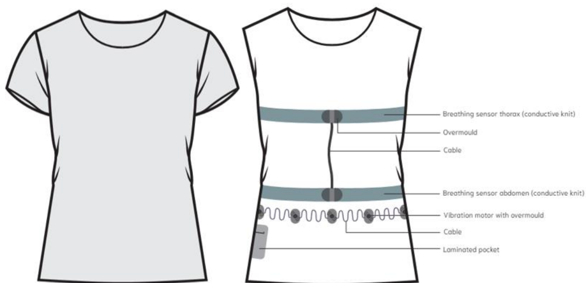
Figure 3. The prototype of the Wearable Breathing Trainer.
