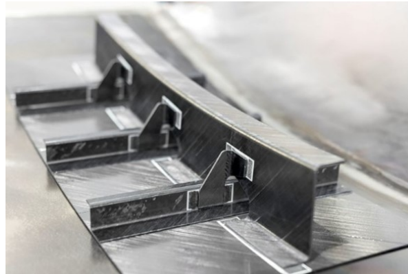
Figure 1.2: Demonstration of a thermoplastic fuselage section, showing a welded stiffened panel.[8]
