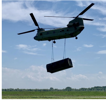
Figuur 30: Container noodmaatregel [Mitchell, 2019].
