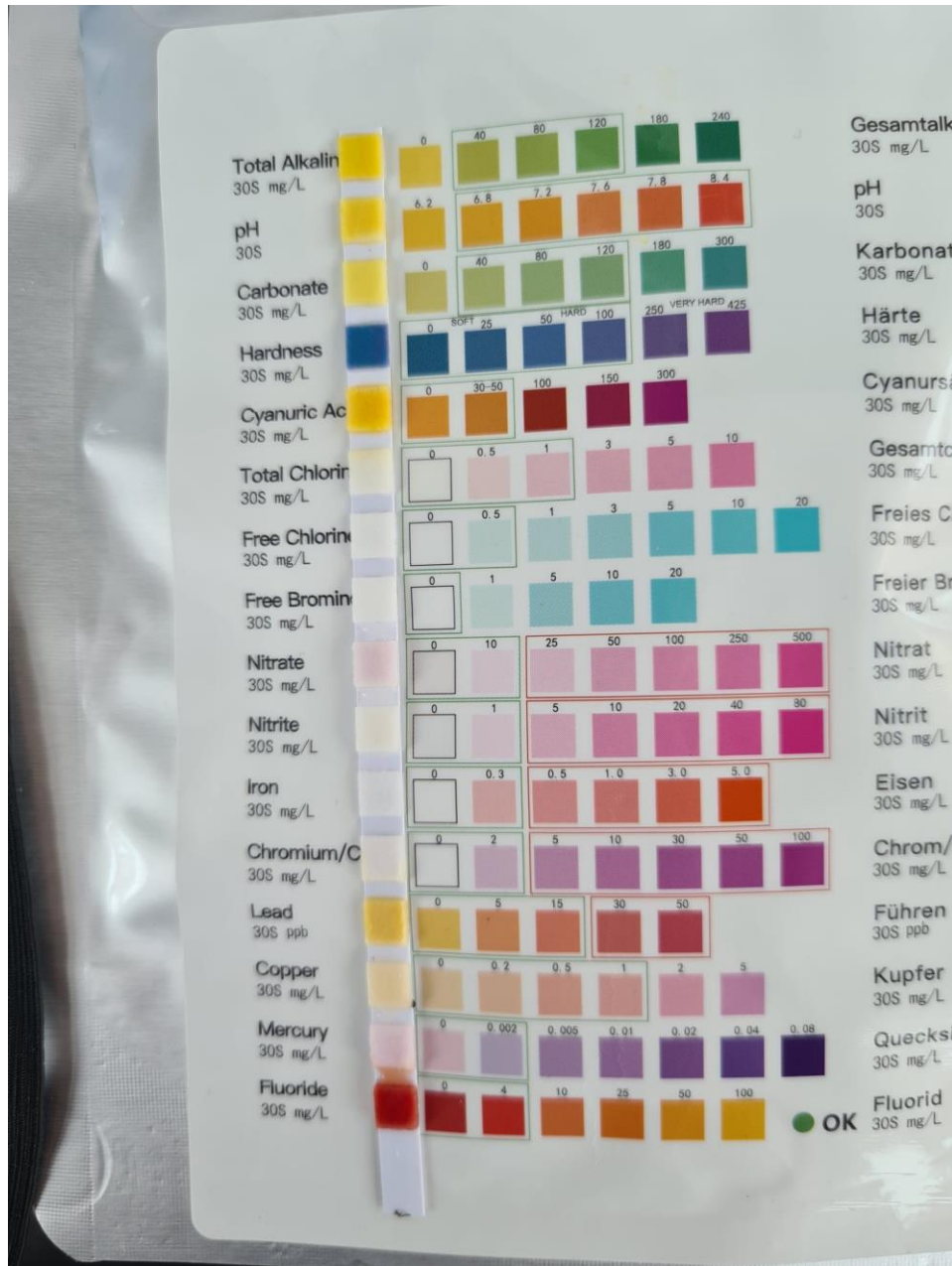
16-Parameter water quality test after filtration.
