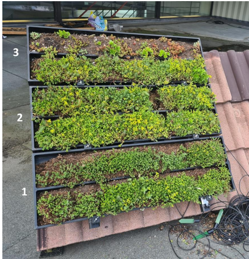
Figure 5. Three numbered modular green panels, labeled 1 through 3, with a total combined surface area of 1 square meter.
