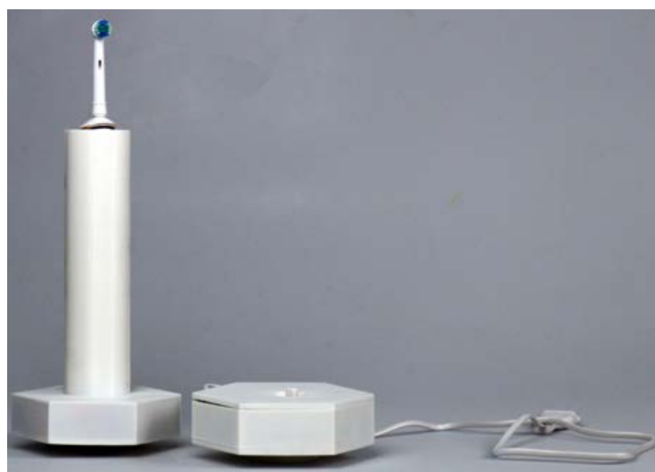
Figure 3.8 TumbleTooth; a toothbrush that rotates as an exercise for hand rehabilitation [18].
