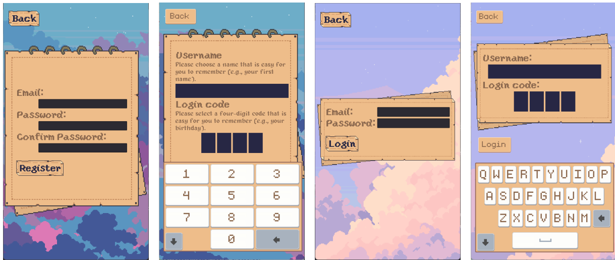
(a) Registration page designed for the prototype. The registration page makes use of the phone's built-in keyboard. (b) New registration page. A keyboard with only numbers allows users to fill out a code. (c) Login page designed for the prototype. (d) New login page. A keyboard with letters allows users to fill out their username.
