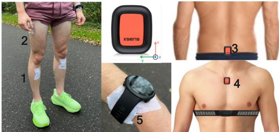
Figure 2 Measurement setup. Sensor placement points: both tibias (1), thighs (2), pelvis (3), sternum (4) and wrist (5), and the sensor coordinate system.
