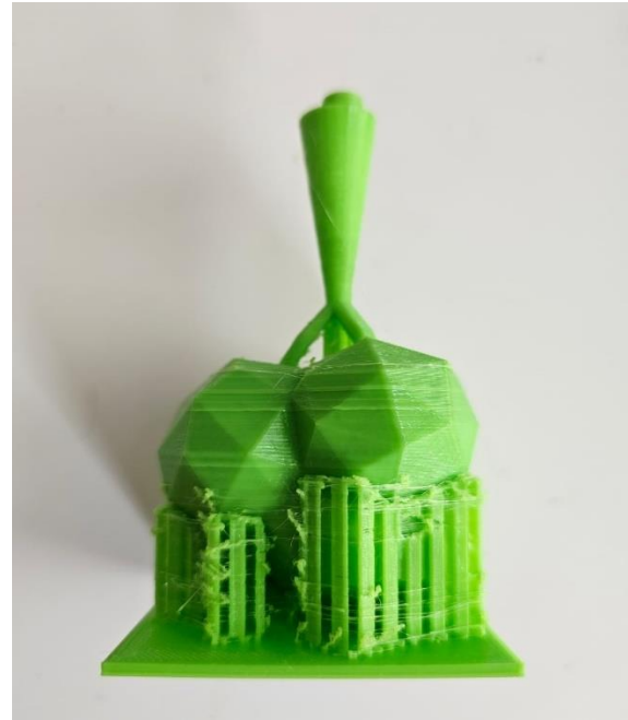
Figure 8, the 3D-print of the upside down plain tree completed with the original supports still attached.
