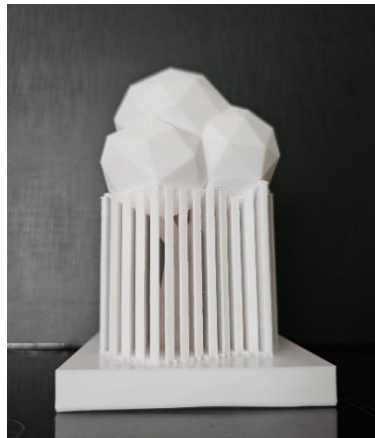
Figure 5, the test 3D-print of the plain tree completed with the original supports still attached.
