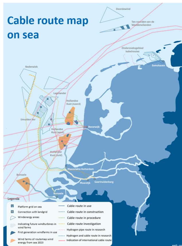
Figure 1: Submarine cable route map with cables from wind farms and between countries. Including current and planned wind farms (COGEA, 2014; Noordzeeloket, 2023b)
