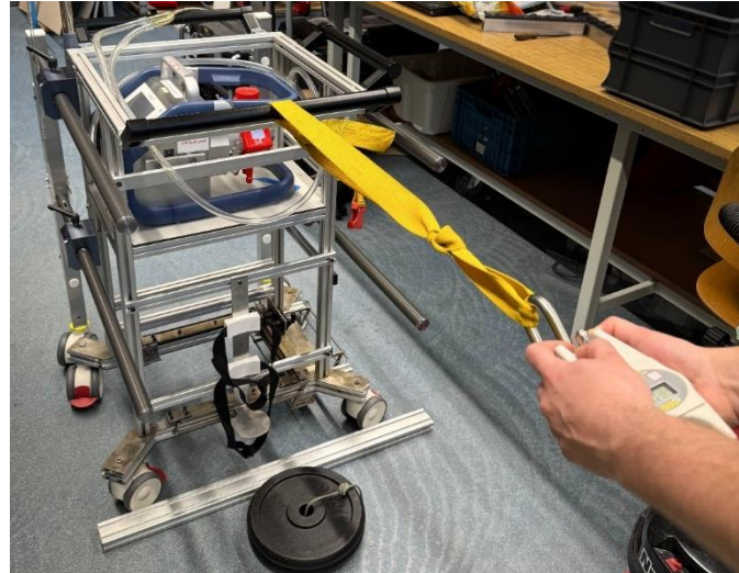
Figure 37: Test setup tipping forces ECMOve V1
