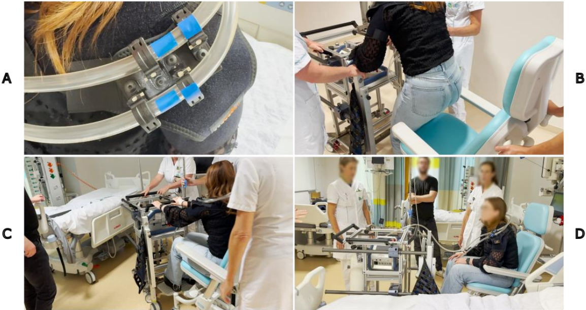
Figure 36: Blood tubing stability test using markers on both the tubing and the connectors (A), Hill-Rom chair for seated patient transport (B) navigating ECMOve and Hill-Rom through ICU (C), ECMOve and Hill-Rom chair next to patient's bed (D).
