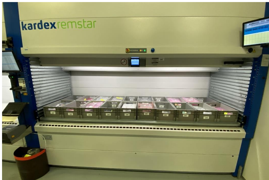
Figure 10: Impression of a retrieved carrier containing B003 boxes
