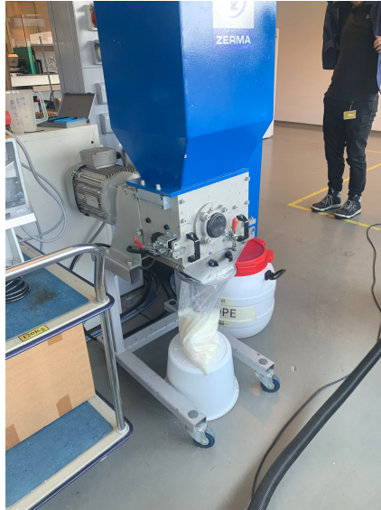
Figure B.1: Granulation of second-time process material with reduction of particle size, screen with 4 mm diameter holes
