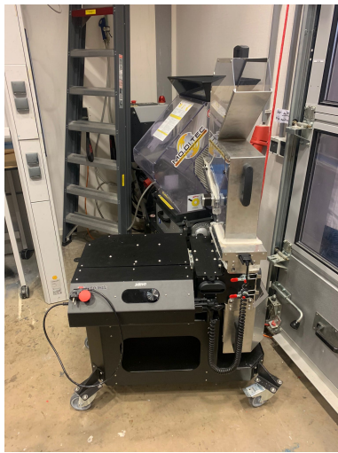
(a) 3Devo shredding machine for making flakes of 3 mm
