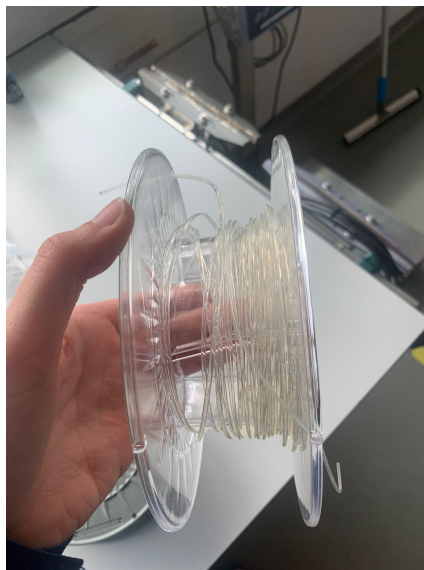
Figure B.4: Results from second recycle protocol at CHILL with the COLLIN. A short filament spooled with air bubbles and inconsistent diameter
