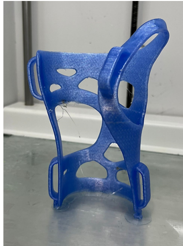
Figure 3.4: The 3DxSplint printed without support structures using recycled PETg material on an Ultimaker S5, employing generic PETg print settings and a print temperature of 230°C
