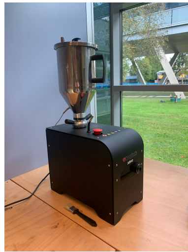
(b) 3Devo drying machine for drying the flakes before filament extrusion.
