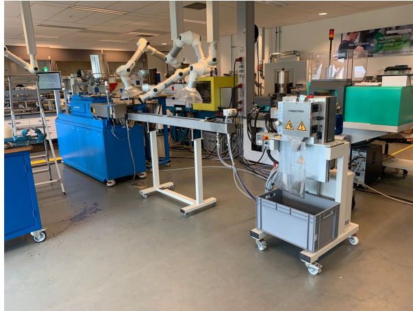
Figure B.6: Filament extrusion on the Corperion extruder left, in the middle the water bath and right the Corperion pelletizer is placed.
