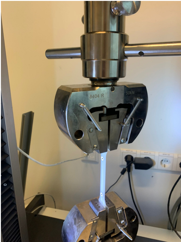
Figure C.5: Tensile test set up with the Zwick/Roell Z020 tensile testing machine.
