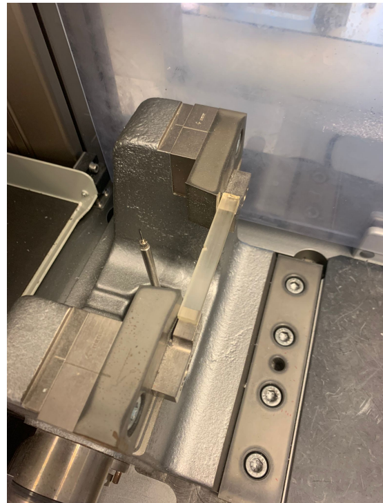
Figure C.7: Alignment of the specimen in the testing machine.
