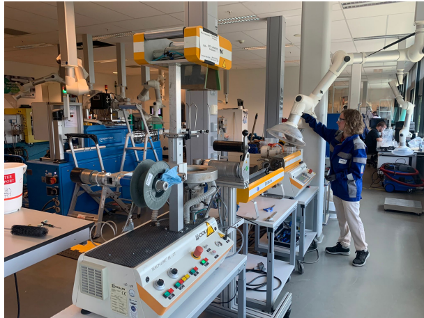
Figure B.3: COLLIN Tech-Line extruder with a water bath
