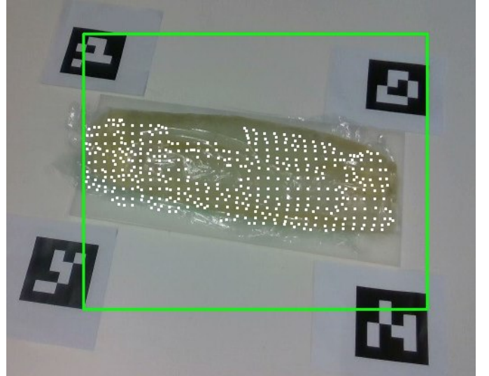
Fig. 4. Four fiducial markers define a Region of Interest (ROI) to help localize the target, in this case a forearm phantom.
