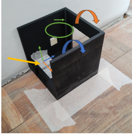
Figure 7: This cube and its marked starting position were used for the sensor calibration measurements. The location of the sensor is indicated by the yellow arrow. Additionally, the sensor's frame is shown. The coloured arcs are the rotations around the corresponding axes ( 90^\circ , 90^\circ and 360^\circ for the x-, y- and z-axis respectively).
