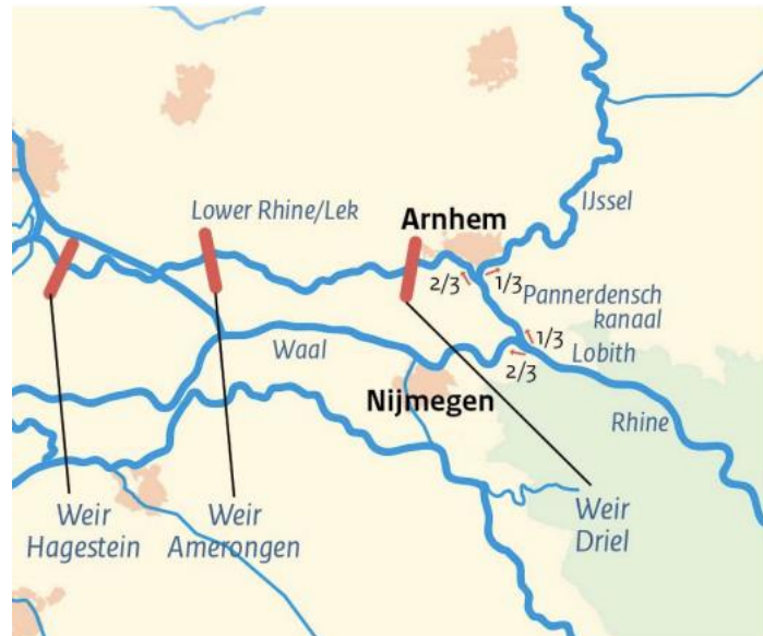
Figure 4 - Distribution of water through the branches of the Rhine, (Water Management in the Netherlands the Kreekraksluizen in Schelde-rijnkanaal, n.d.)
