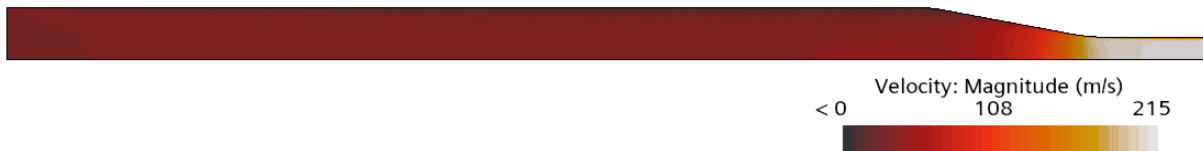
Figure 5.1: Velocity Field for Single-Phase Steam Passing Through a Nozzle.
