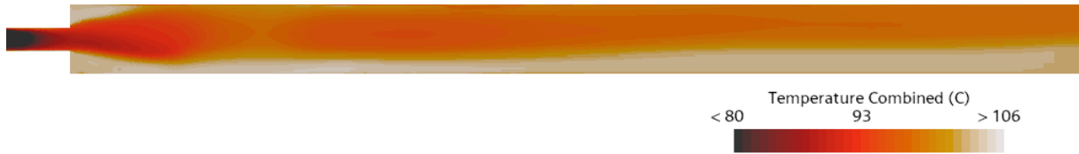
Figure 5.13: Temperature Distribution in the Outlet Region.
