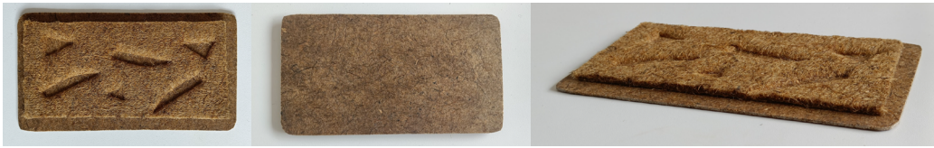
partially pressed layer on hard pressed layer
