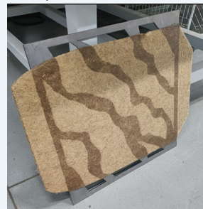
Figure 48 Hemp sticking to steel
