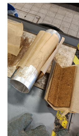
by only putting mass on pre-preg during baking
