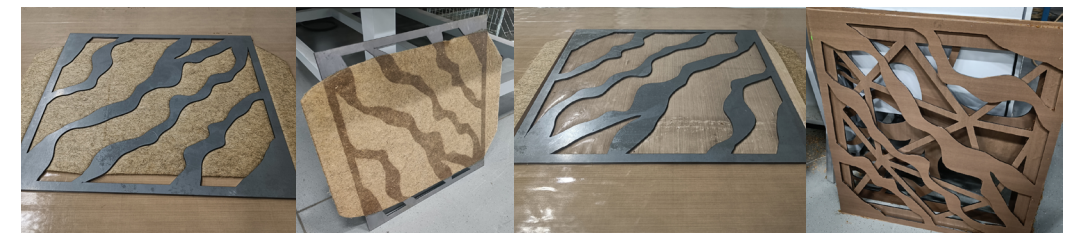
Without coating or Teflon cloth, sample sticks to steel, with Teflon cloth
