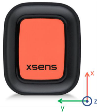
(a) DOT sensor coordinate system [53]
