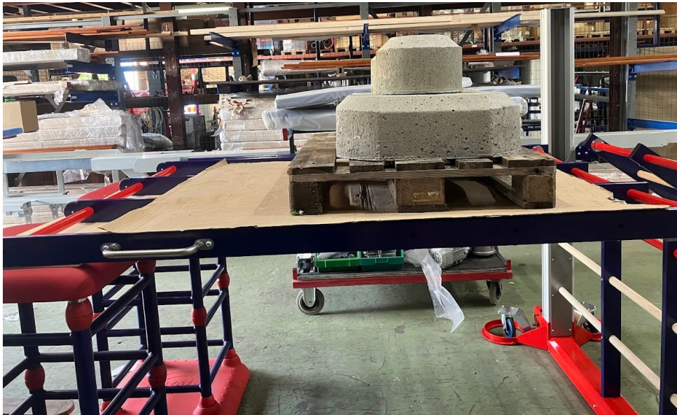
Figure 60: Load test of climbing frame
