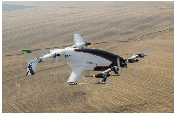
FIGURE 1.1 – The Airbus A3 Vahana, a quad tiltwing eVTOL demonstrator aircraft (sUAS News, 2019).
