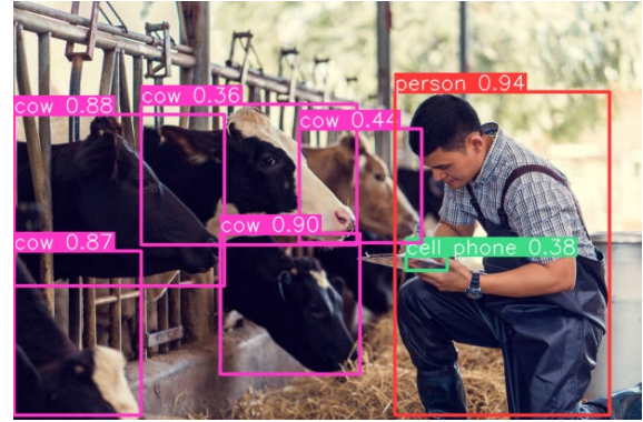
Fig. 5: Example of YOLO-based object detection output from an image of a farmer with cows. The output shows the bounding boxes of the detected objects, the classification of these objects, and the confidence for these classifications.
