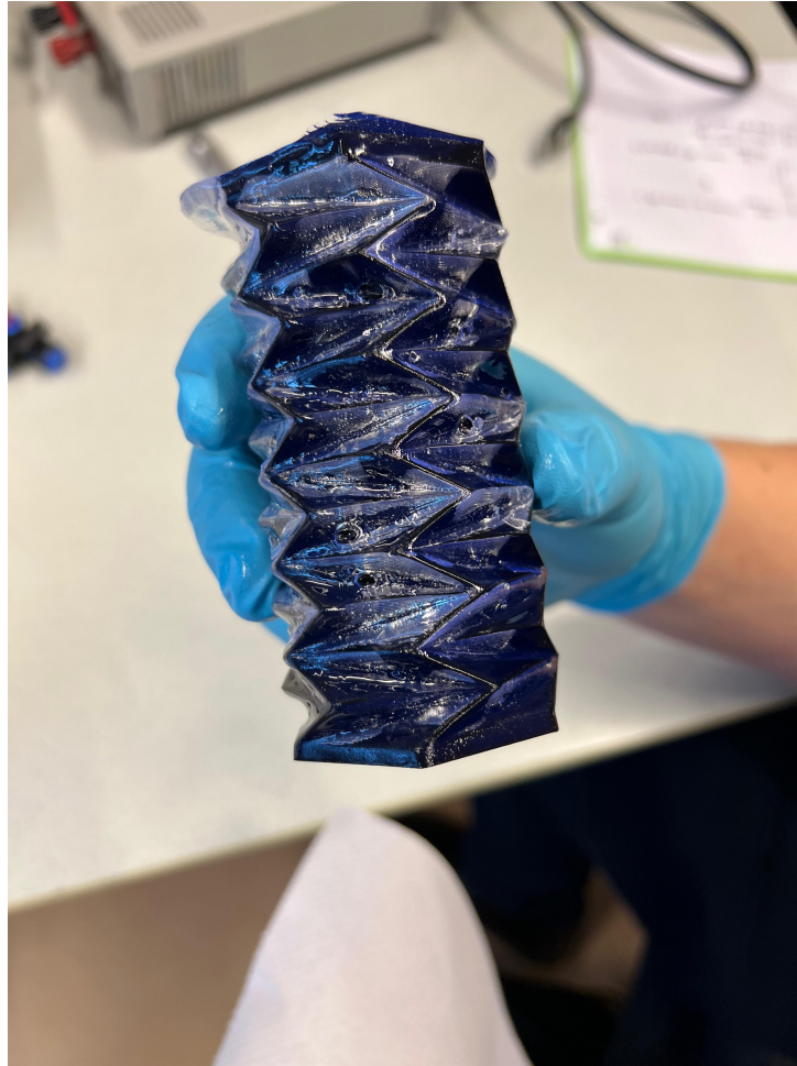
Figure 23: Actuator with elastic resin coating
