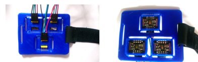
Figure 2: On the left the top view of the sensor holder is shown holding three MAX30102 sensors. On the right the bottom of this is shown.
