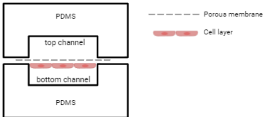
Figure 2: Cross-section view of a standard BBB-chip, with from top to bottom the top part including the top channel, the porous membrane, the iPSC monolayer, which is attached to the membrane and the bottom part including the bottom channel. The schematic is not to scale.
