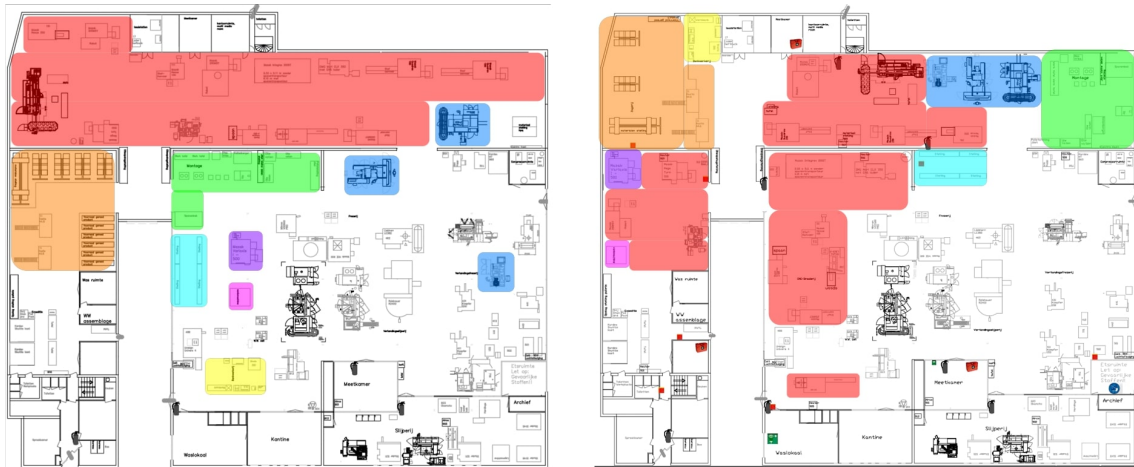
FIGURE 59: Redesigned layout (left) and current layout (right), indicating which other departments and machines have a changed location by color: lathe department (red), sawing department (orange), bench-working department (yellow), assembly department (green), storage racks (light blue), gear milling machines (dark blue), milling machine (purple) and spark-erosion machine (pink).
