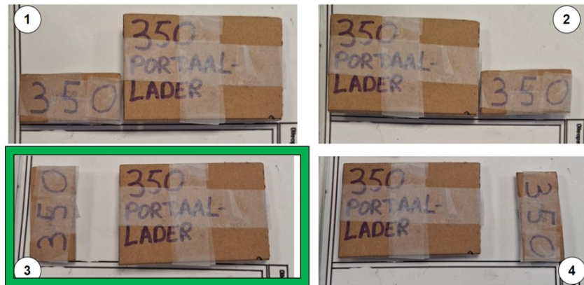
FIGURE 52: Carton board on whiteboard is used to check dimensions and orientations of machines to be placed. Option 3 is chosen.
