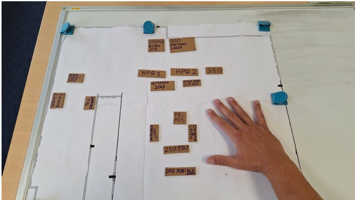
FIGURE 34: First version, complete blank layout was printed and put on whiteboard together with scaled cartons representing machines with their names written on. Machine locations are from the current layout. Hand for scale.
