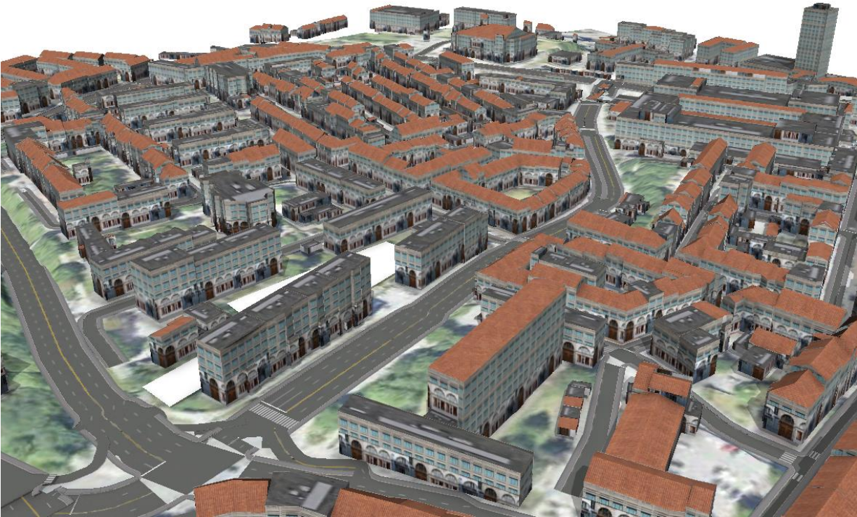
Figure 43: Adding texture to the building facade using the CGA rule for Zurich City. Source: Author, 2024.
