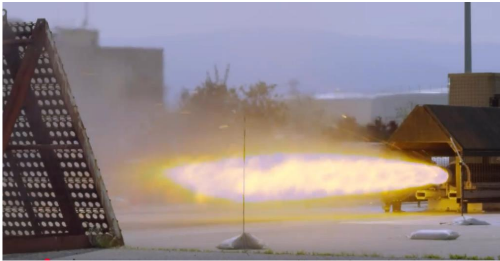
Figure 21: Paraffin Powered Rocket Engine developed by NASA at the Ames Research Center [41]
