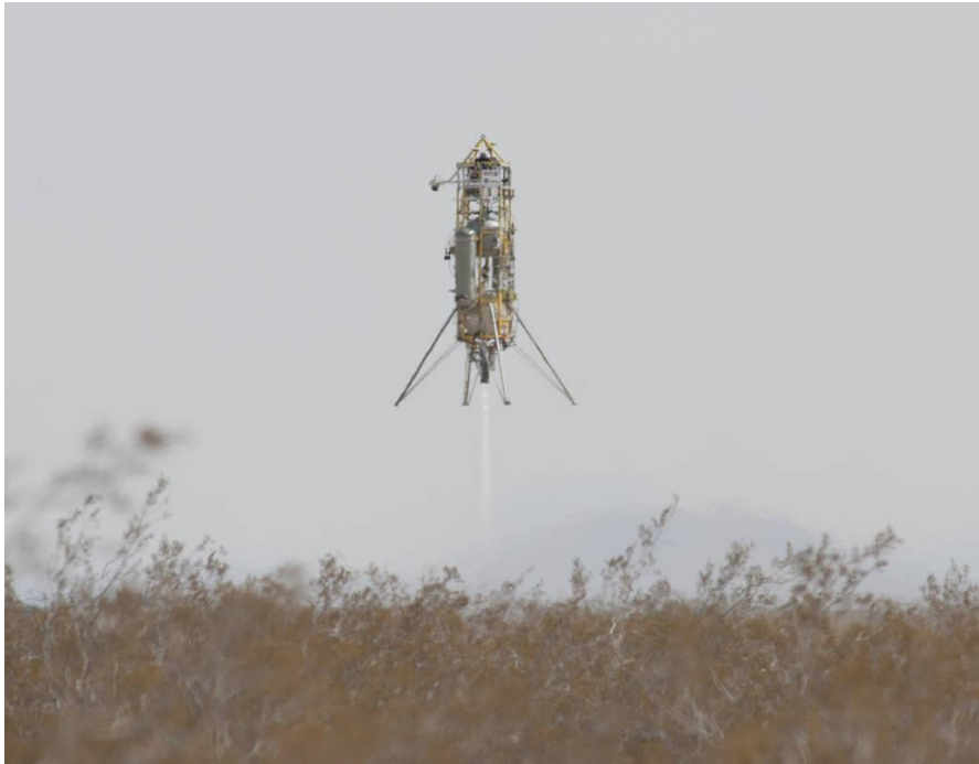
Figure 2: Masten's Xombie Space-Access technology demonstrator used by NASA to develop the GENIE GNC system [7]
