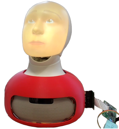
Figure 6: The finished touch-sensitive interface as shell around the Furhat.
