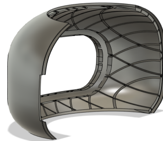
(c) Design of the insight of the front of the shell, showing the other half of the connection mechanism.
