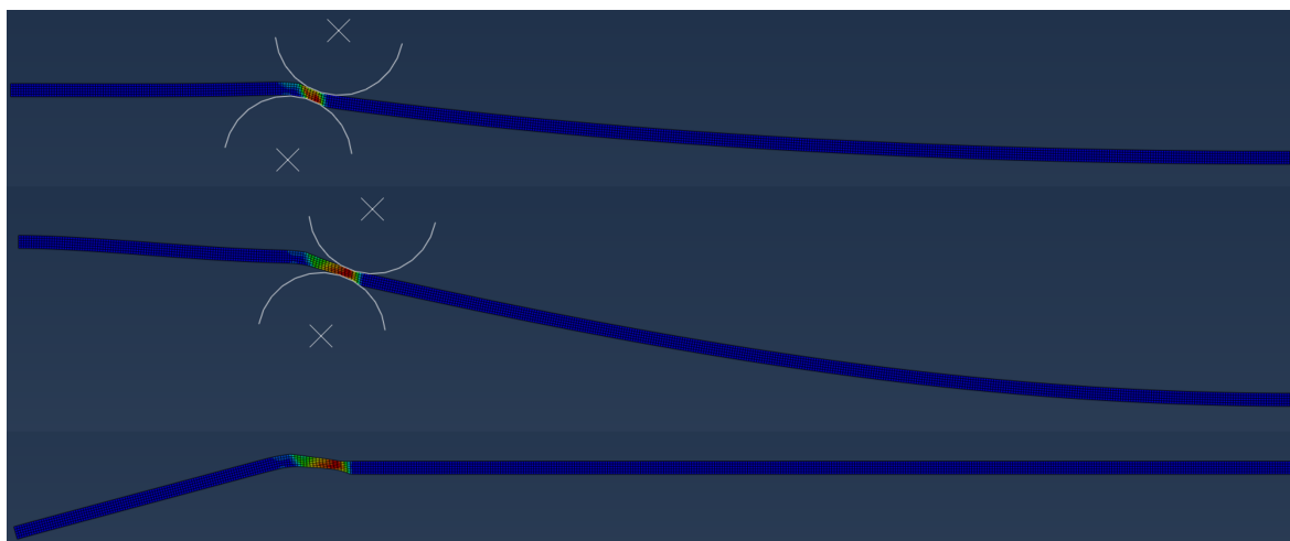
Figure 4.14: PEEQ of the multi-pinch forming for zero tool angle. First two pictures are at the end of the third and of the tenth pinch, respectively. The last picture is after the clamps have been removed. The darkest red indicates a large strain of 50%.
