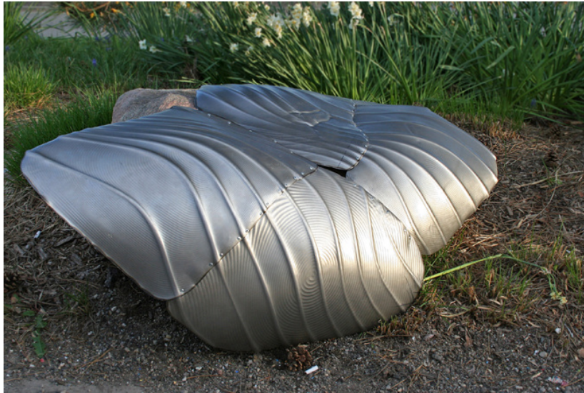
Figure 1.4: Four individually formed parts using ISF. Note the forming lines on the parts, caused by incremental forming [5]
