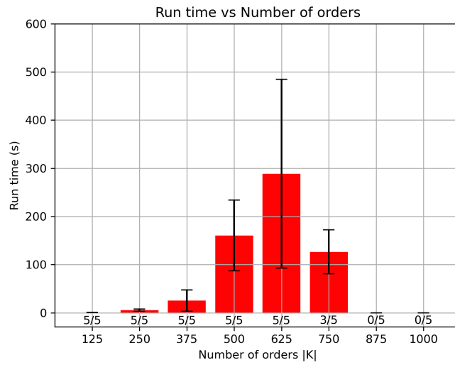
FIGURE 13: The average run time of the mixed-integer program over 5 instances for different numbers of orders |K| . The fraction below each bar represents the number of times the mixed-integer program was able to find an optimal solution within the 10-minute time limit.
