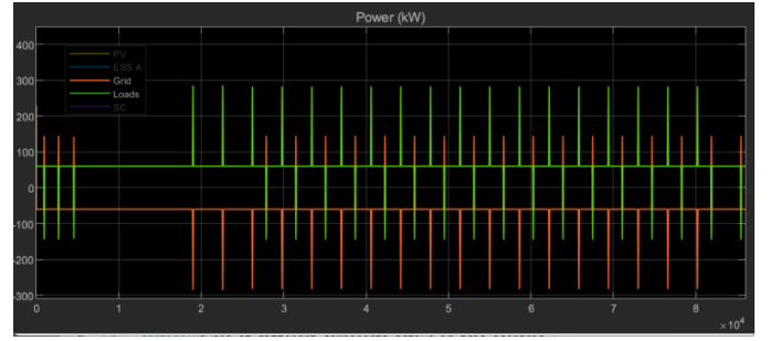
Fig. 15. Powers of different components active in the Base Case scenario. The x-axis is time for 24h and the y-axis corresponds to Power (kW).
