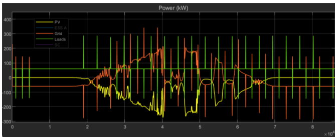
Fig. 17. Powers of different components active in the PV Only scenario, when its a cloudy day. The x-axis is time for 24h and the y-axis corresponds to Power (kW).
