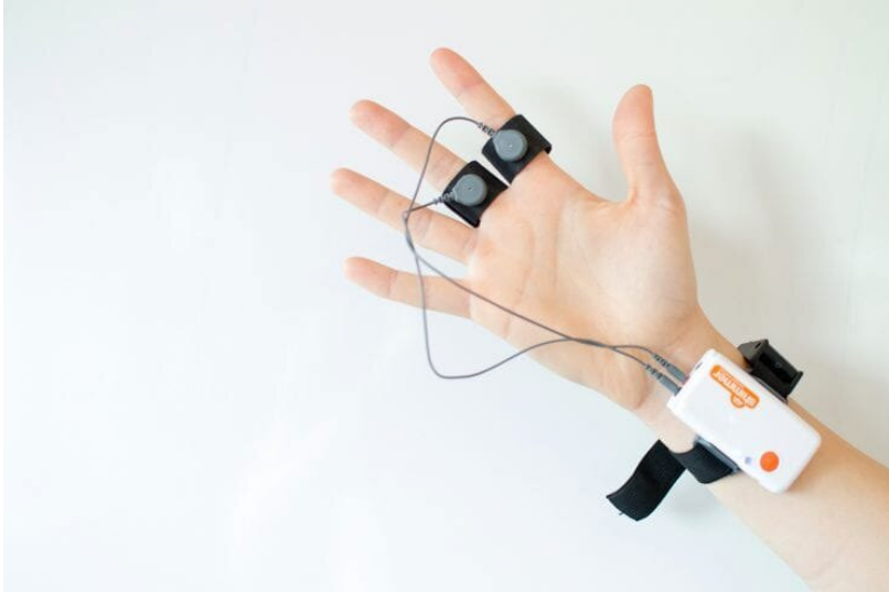
Figure 5.1: Consensys Shimmer3 bundle, which was used in this study to collect physiological data such as Galvanic Skin Response (GSR) and heart rate [39].
