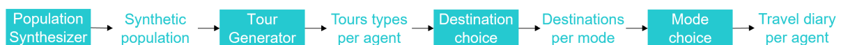
FIGURE 1.2: Schematic overview of the four stages in the current travel demand modelling framework in Octavius. The blue boxes represent the population synthesizer and the choice models, whereas the in- and outputs to the stages are represented as blue text without background.
