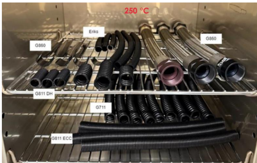
Figure 49: Test #2 aging setup inside the Thales oven
