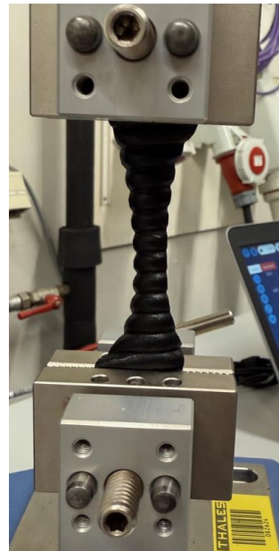
Figure 35: PTFE sample clamping
