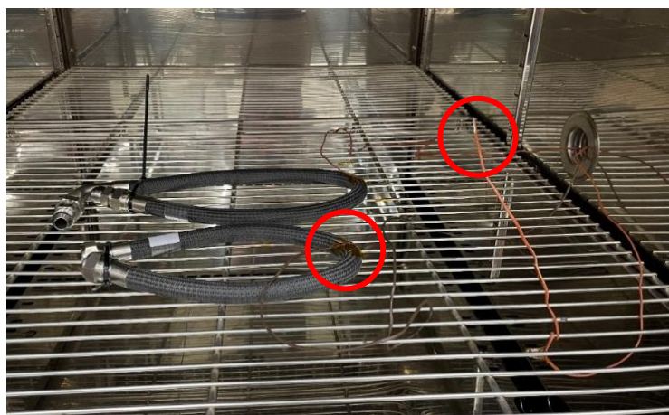
Figure 46: Temperature cycling test setup; hoses placed inside
