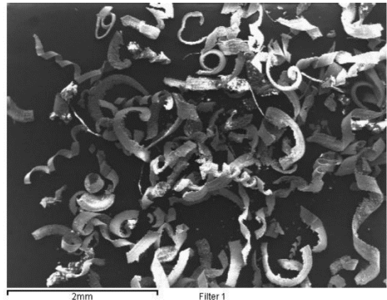
Figure 30: SEM picture of sharp metal parts inside operational Dowcal coolant fluid
