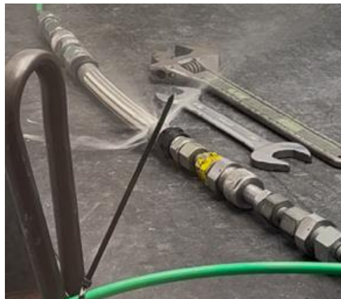
Figure 63: Screenshot of moment of failure during the burst pressure test - unaged G860 hose
