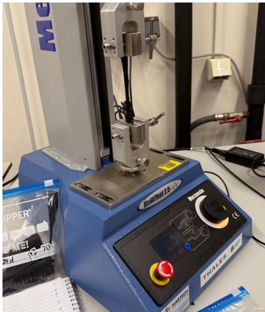
Figure 34: Tensile test setup
