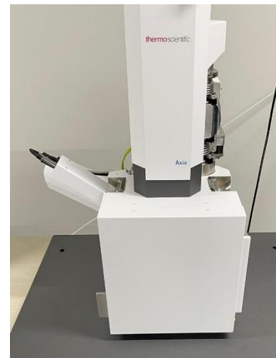
Figure 32: Microscopic SEM analysis machine: Thermoscientific Axia
