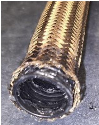
Figure 64: G860- 250C-24d Coupling removed after burst
