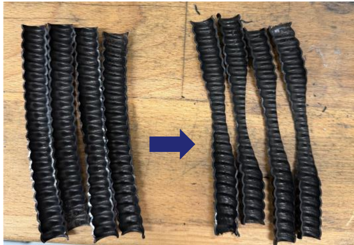
Figure 43: Sample preparation - cutting for tensile tests
