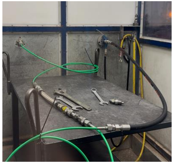
Figure 39: Burst pressure test setup
