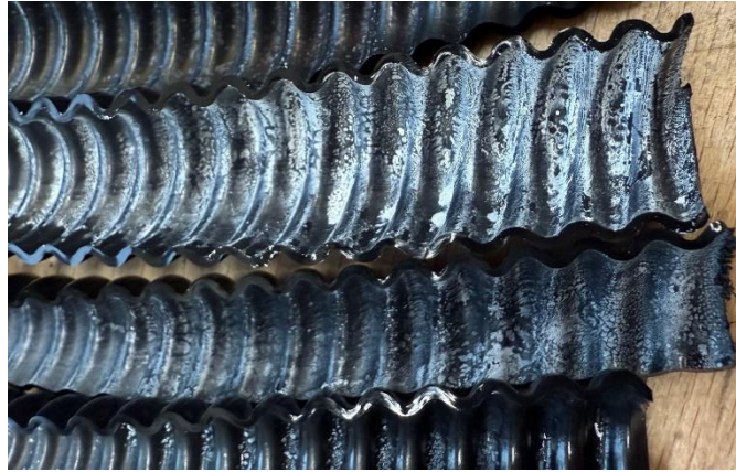
Figure 66: Inside surface of the G711 REF DH hose - Dowcal residue
