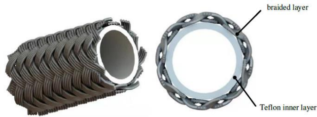
Figure 5: 3D model of a general PTFE hose construction
