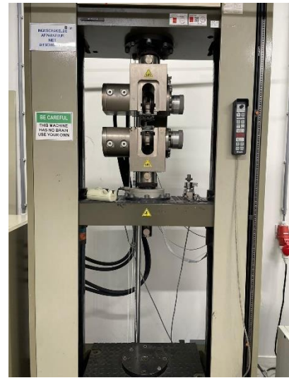
Figure 36: Tensile test setup; heavy
