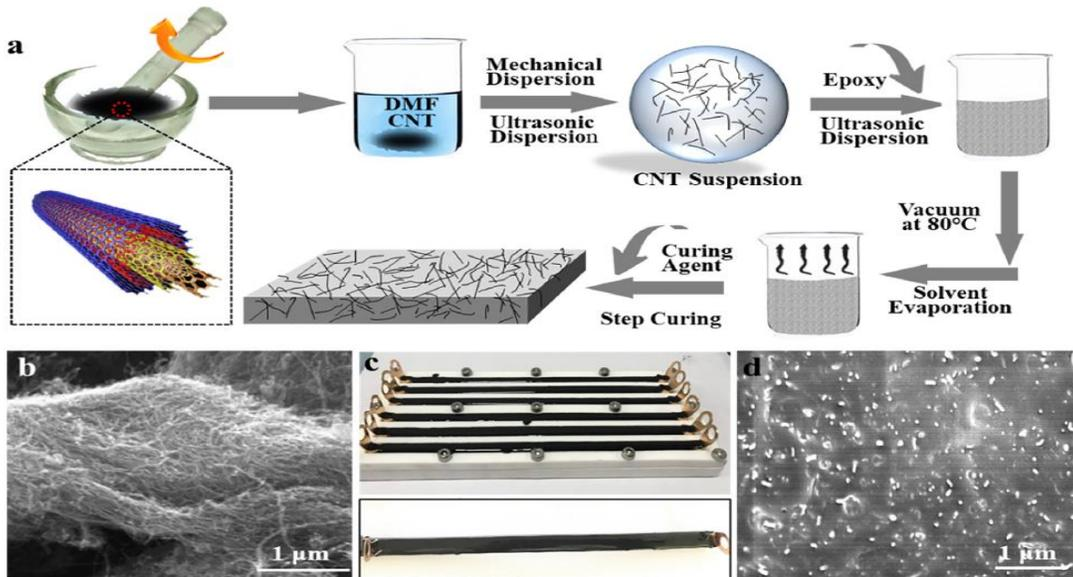
Figure 32: Preparation and morphology of nanocomposites. a. Schematic diagram of the key steps in fabricating the composites strain sensor b. SEM image of aligned MWCNTs (Xin, Liang et al. 2020).
