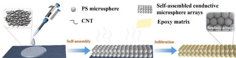
Figure 33: Schematic of the preparation process of sensing nanocomposites (Su, Jiao et al. 2024).
