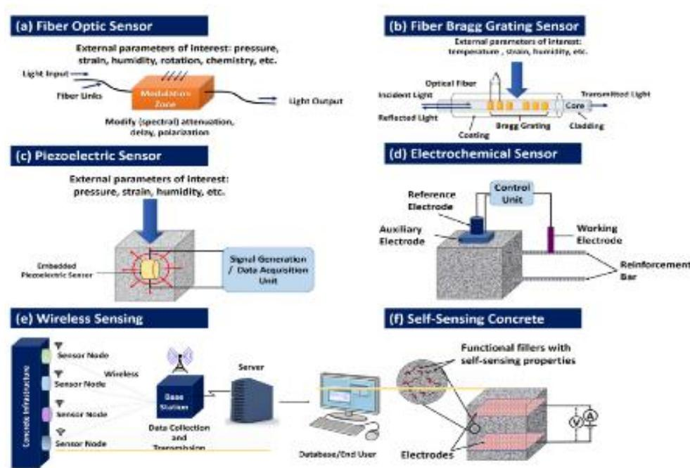
Figure 22: Illustration of a sample (a) optical fiber sensor, (b) fiber Bragg grating sensor, (c) piezoelectric sensor, (d) electrochemical sensor, (e) wireless sensor system, and (f) self-sensing concrete (Taheri 2019).
