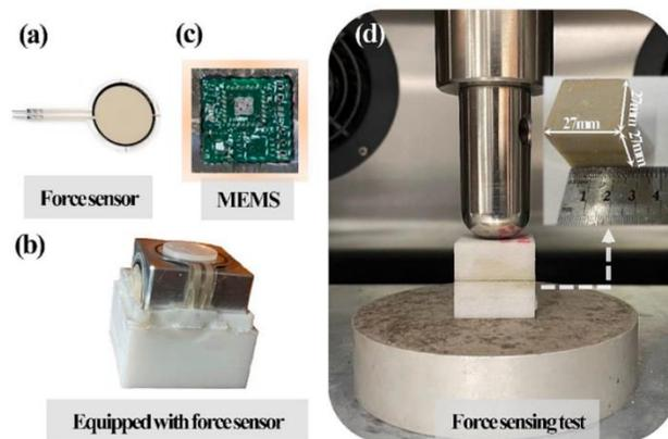
Figure 20: Smart Aggregate and its force sensing test (Li, Sha et al. 2023)
