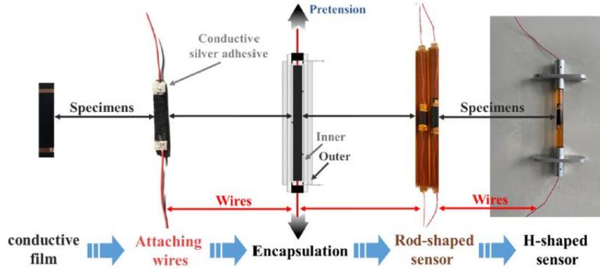
Figure 34: Encapsulation process of self-sensing nanocomposites with enhanced durability and compatibility for engineering applications (Su, Jiao et al. 2024).
