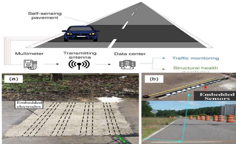
Figure 25: Self-sensing road pavement and Self-sensing configurations: (a) bulk and (b) array arrangements
