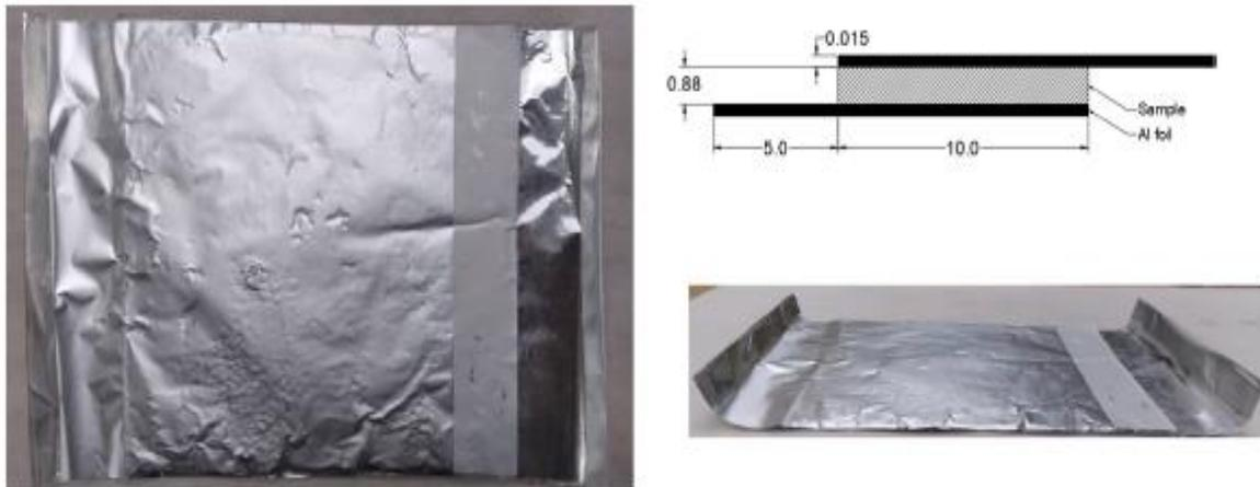
Figure 23: Photographs of the capacitor with pitch-matrix composite sandwiched by aluminum foil (Ozturk and Chung 2021).
