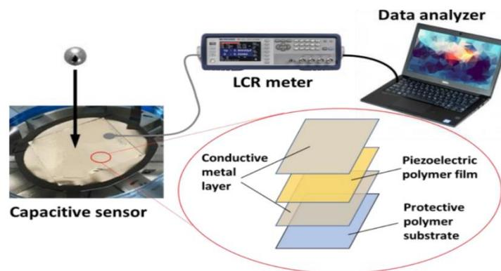
Figure 10: Film form of polymer piezoelectric sensors (Arkema).
