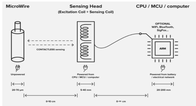
Figure 14: Operational Structure of RVmagnetics Diagram
