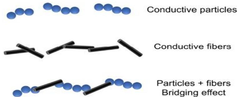
Figure 24: Combining conductive particles and fibers (Gulisano, Jimenez-Bermejo et al. 2024).
