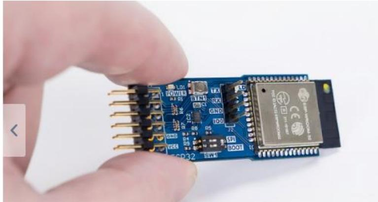
Figure 11: ESP32 Wireless Communication Module (Espressif 2024)F.
