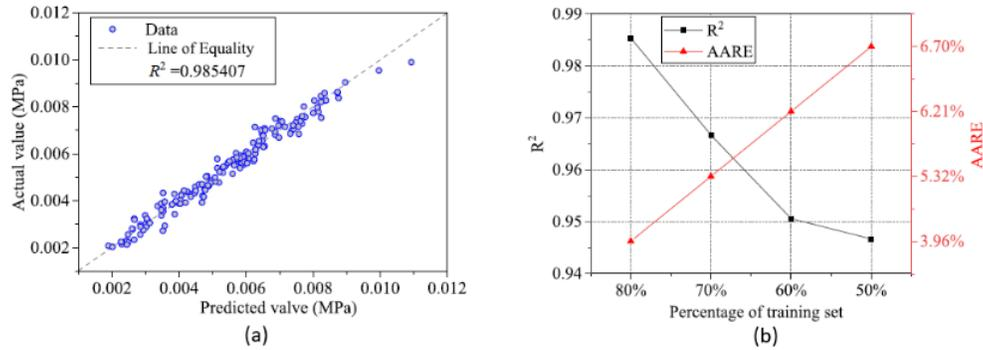
Figure 28: Correlation between actual ABAQUS FE values and Kriging predictions (a), Variation in prediction accuracy of spherical models with the proportion of the training set (b) (Wang, Han et al. 2022).
