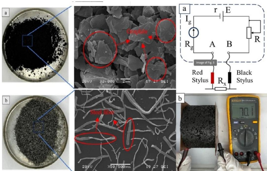
Figure 26: Conductive additives (a. graphite; b. steel fiber). Resistance meter model and test procedure (a: resistance meter model; b: test procedure) (Li, Hu et al. 2024)
