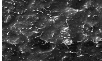
Figure 30: : Scanning Electron Microscopy of carbon nanotube-modified epoxy resin
