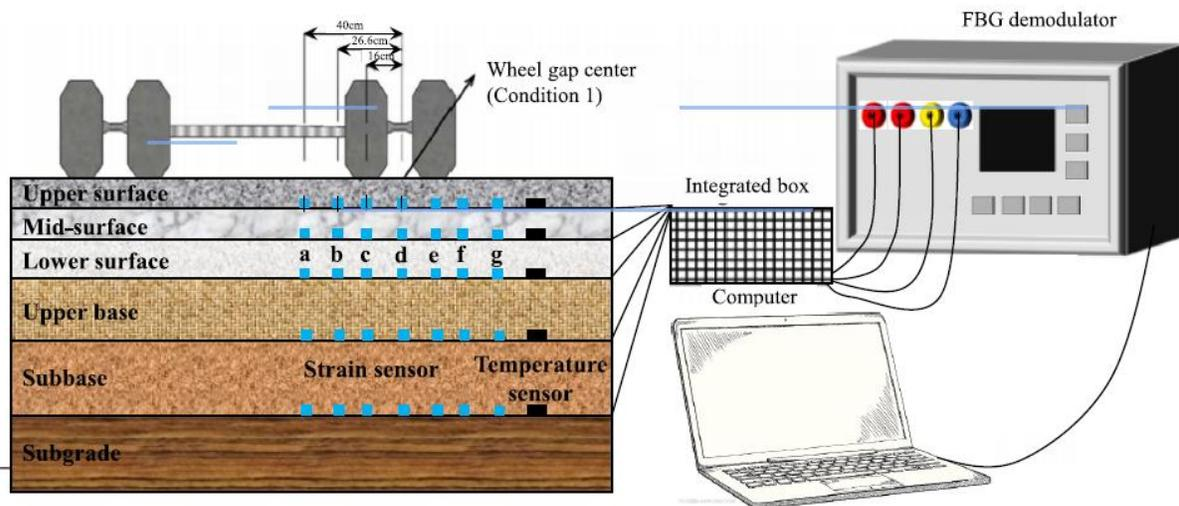
Figure 21: Assembled FBG sensor and Sensor layout in road structure (Wang, Han et al. 2023).
