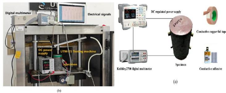
Figure 29: Resistance measurement of MWCNTs/Epoxy mixtures (Huang, Wang et al. 2024).
