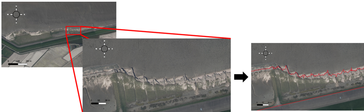
Figure 3.2: Example of the determination of the marsh edge on the PDOK image of 2023. The red line is the digitization of the marsh edge.
