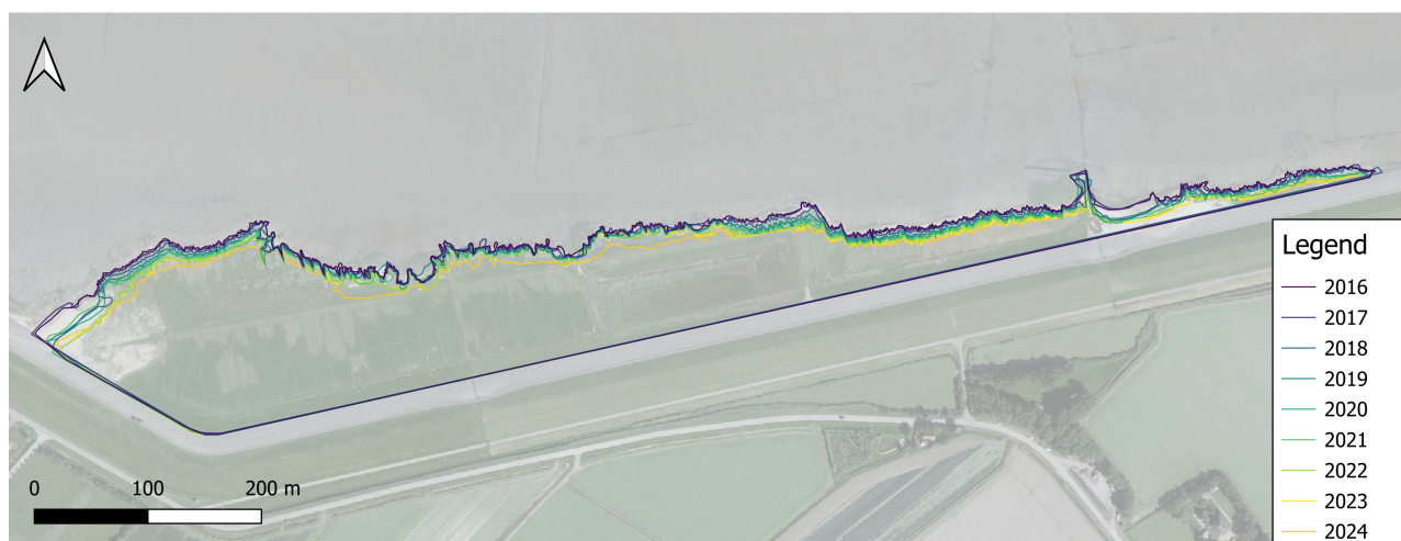
Figure 4.1: Map of the Wierum marsh edge retreat from 2016 until 2024 using PDOK data. As background map the aerial image of 2016 is used.
