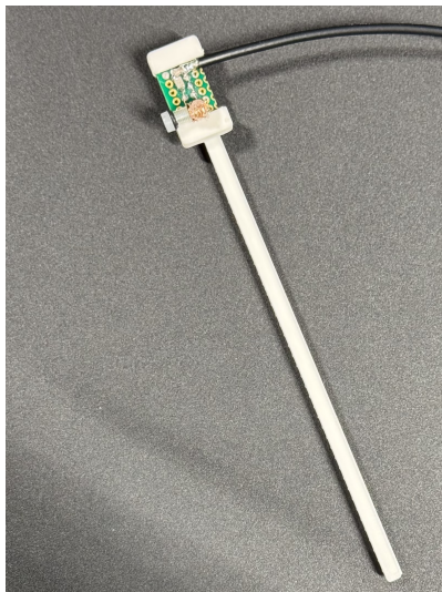
Figure 3.10: 3D-printed coil holder to attach the RF microcoil to MAMRI as surrogate needle
