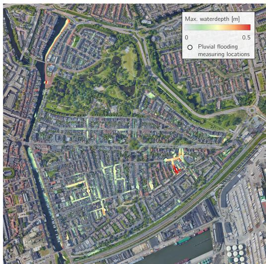
Figure 16: Maximum depth of pluvial flooding after a T2 2050 composite rainfall event. The eight measuring locations are the ones shown in Figure 7. Values of the measurements are given in Table 9.
