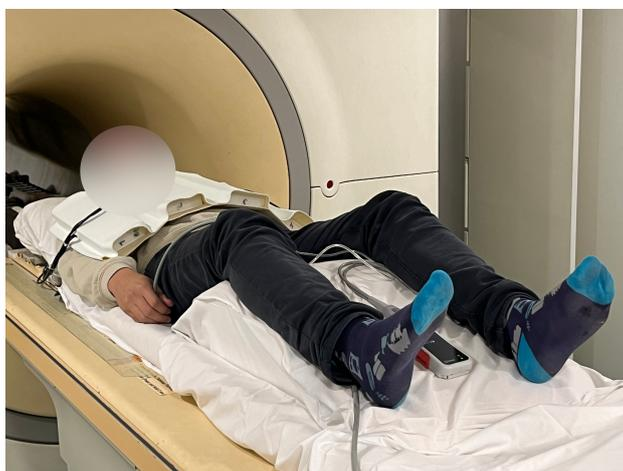
**Figure 5:** Measurement setup of in vivo MRSI scans at 7T. The coils were placed below and on top of the thorax. The air bag of the respiratory sensor was placed on the stomach using a belt. The respiratory sensor itself was placed between the legs. Volunteers were positioned feet first.
