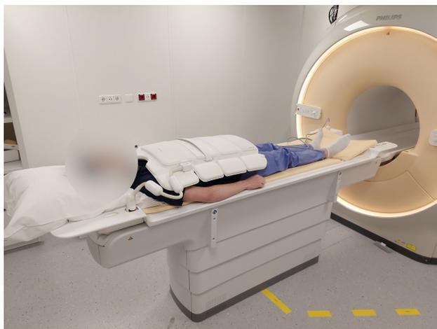
**Figure 4:** The experimental setup for experiment 1 at the 1.5T scanner with a volunteer out of the bore. The abdominal coil is placed on the thorax. The volunteer was positioned feet first.
